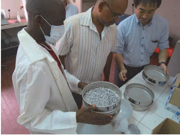
Photo 2.3-22 Crushing and Sieving of Rocks for Zircon Separation
