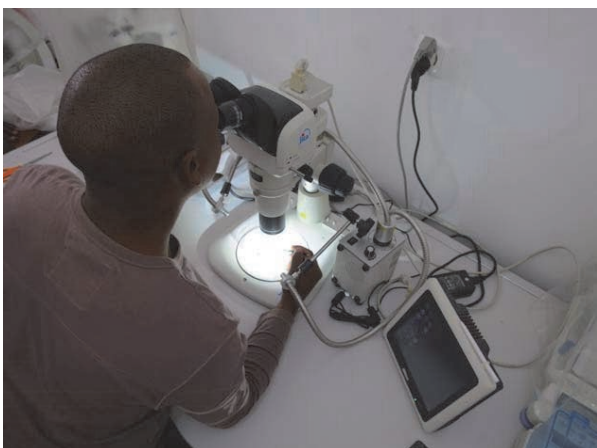
Photo 2.3-30 Mineral Separation of Zircon by Stereomicroscope
