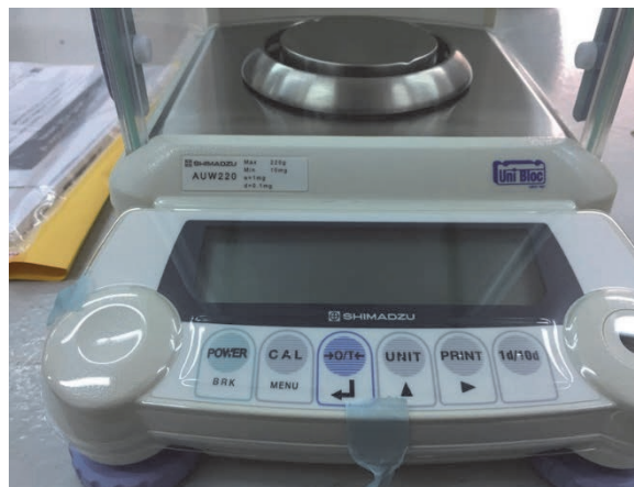
Photo 2.2-5 Electronic Analytical Scale: 2 sets (SHIMADZU AUW220)
