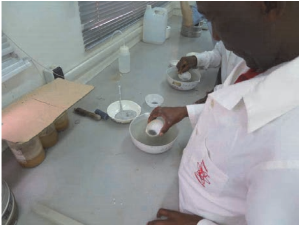
Photo 2.3-23 Elutriation and Drying of Selected Samples by Sieving
