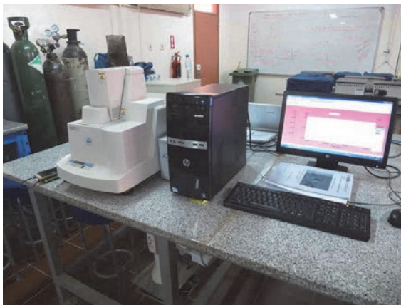
Simultaneous Differential Thermogravimetric Analyzer (SHIMADZU DTG-60)
