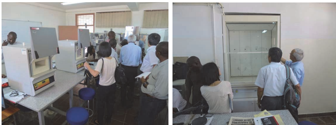
Photo 2.1-14 Muffle Furnaces and Cupellation Furnace (left) and Draft (right)
