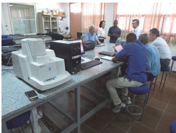
Practical Training for Reaction Rate Analysis of Coal Samples using Donated Simultaneous Differential Thermogravimetric Analyzer in ISPT
