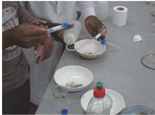
Photo 2.3-29 Results of Heavy Liquid Mineral Separation and Preparation of Samples for Zircon Separation
