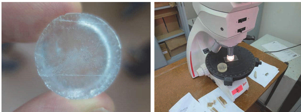
Photo 2.3-31 Preparation of Polished Section for the Separated Zircon
