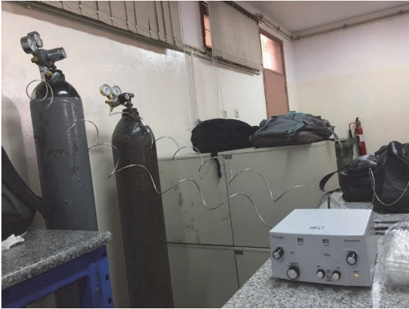
Photo 2.2-23 Conduit Tube for Carrier Gas (5m)
