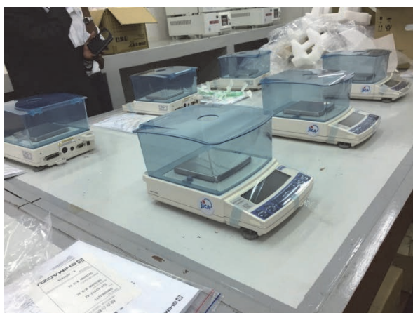
Photo 2.2-7 Electronic Analytical Scale: 3 sets (SHIMADZU UW1020H)
