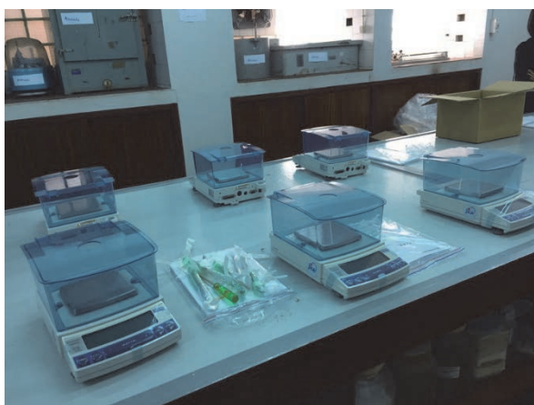
Photo 2.2-6 Electronic Analytical Scale: 3 sets (SHIMADZU UW420H)
