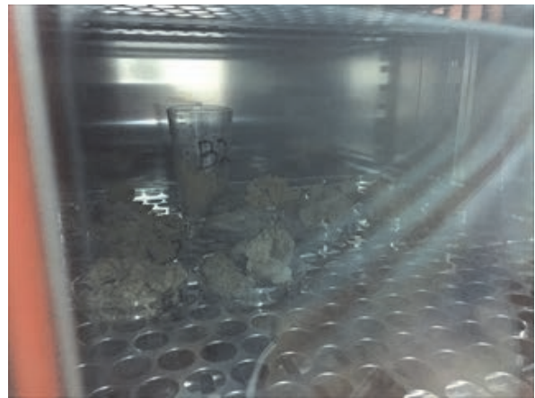
Photo 2.3-18 Usage Condition of Donated Equipment; Oven (for drying of separated clay minerals)
