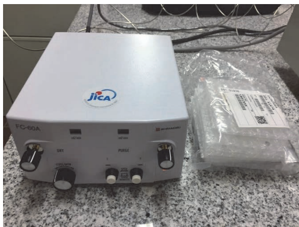
Photo 2.2-21 Atmosphere Control Part (SHIMADZU FC-60A)
