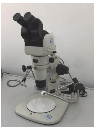
Photo 2.2-2 Stereo Microscope (binocular scope) and Illumination Device (Nikon SMZ1270 TRG-PS32)
