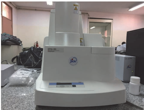
Photo 2.2-19 Simultaneous Differential Thermogravimetric Analyzer (SHIMADZU DTG-60)
