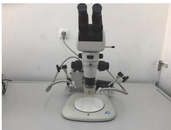
Photo 2.2-2 Stereo Microscope (binocular scope) and Illumination Device (Nikon SMZ1270 TRG-PS32)
