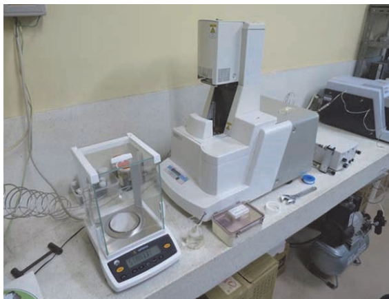
Photo 2.3-39 Practical Training by using Simultaneous Differential Thermogravimetric Analyzer at the Short-term Training in Japan
