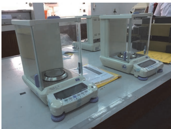
Photo 2.2-5 Electronic Analytical Scale: 2 sets (SHIMADZU AUW220)
