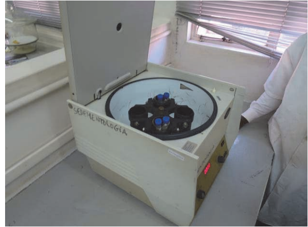
Photo 2.3-28 Preparation of Heavy Liquid (SPT) and Heavy Liquid Mineral Separation by Centrifugal Separator
