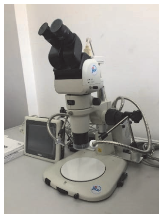
Photo 2.2-1 Stereo Microscope (trinocular scope), Illumination Device and Digital Camera (Nikon SMZ1270 TRG-DSL32-POL)
