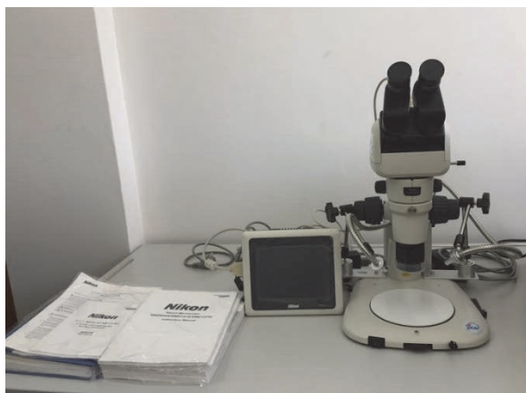
Photo 2.2-1 Stereo Microscope (trinocular scope), Illumination Device and Digital Camera (Nikon SMZ1270 TRG-DSL32-POL)
