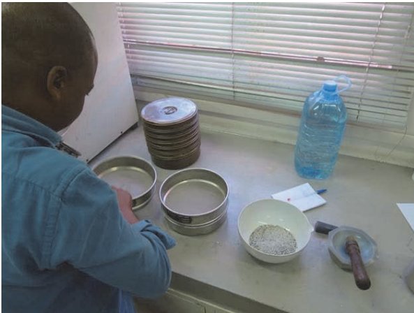
Photo 2.3-27 Preparation of Separation by Sieving and Panning of Pulverized Rock
