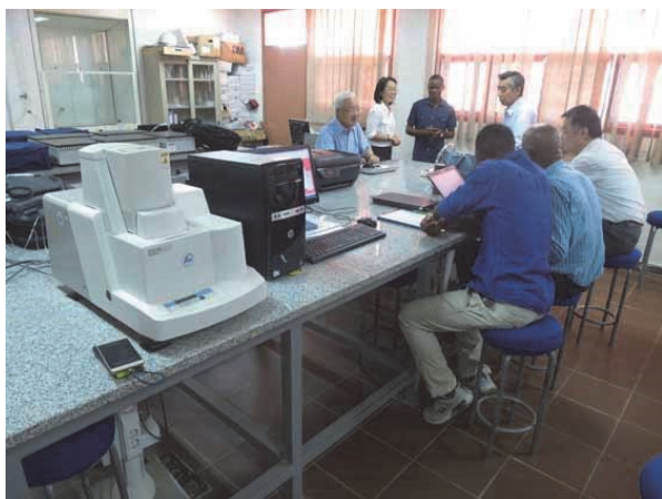
Photo 2.3-58 Instruction of the Velocity Analysis Method by Simultaneous Differential Thermogravimetric Analyzer
