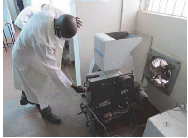
Photo 2.3-22 Crushing and Sieving of Rocks for Zircon Separation
