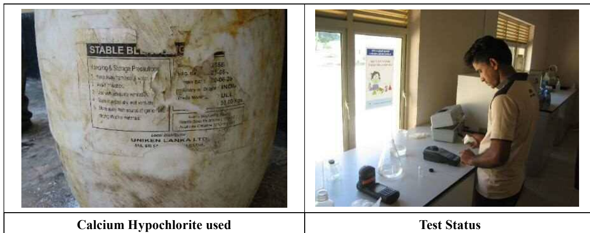
Photo 3-9 Chlorination Test for No.3 SSF Treated Water
