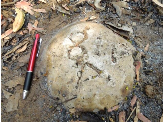
Enlarged photo of the survey beacon set in the cadastral area. It is made from concrete with a diameter of approximately 20 cm without survey nails
