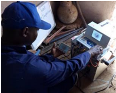
Investigating the inside of a well using a borehole camera
