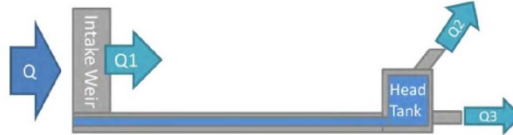
Figure 6-3-4 Image of Calculation Method for Diversion Flow Rate
