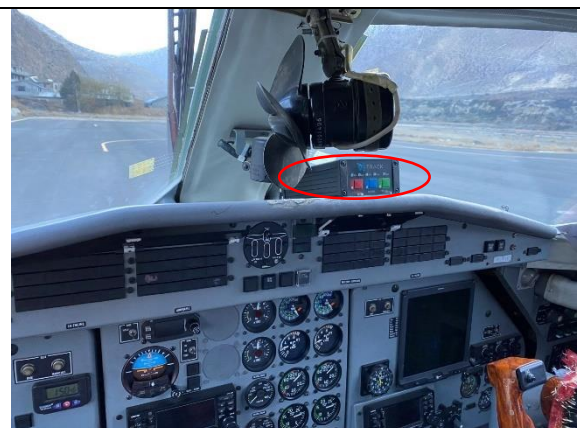
Photo 3.3-9 Summit Air, L410 Cockpit V2 tracker transmitter installed
