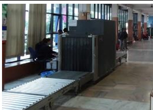
Photo 3.5-7 Checked-in luggage X-ray scanner
