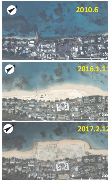
Fig. 13. Change in Beach Condition (Upper: Before Reclamation, Middle: Before Groin Construction, Lower: After Groin Construction).
