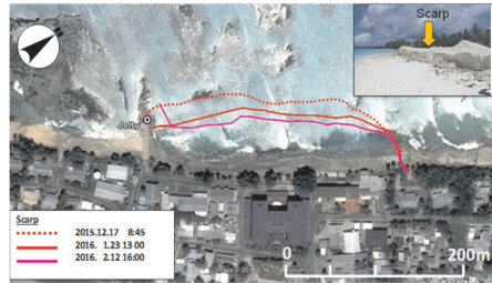
Fig. 12. Change in Shoreline at the Reclamation Area.
