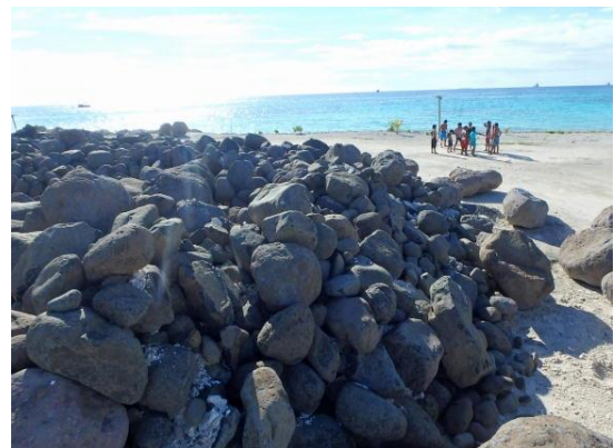
Figure 17.3.8 Armor Rock from Nauru (The Government of Tuvalu Reclamation Project)
