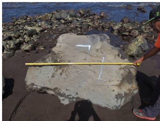
Figure 9.5.8 Example of Armor Stone at Quarry Site
