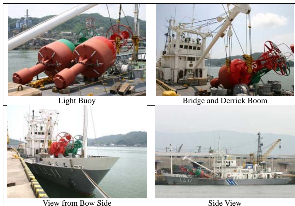
Photo 4-7 Buoy Handling by Anchor vessel in Japan
