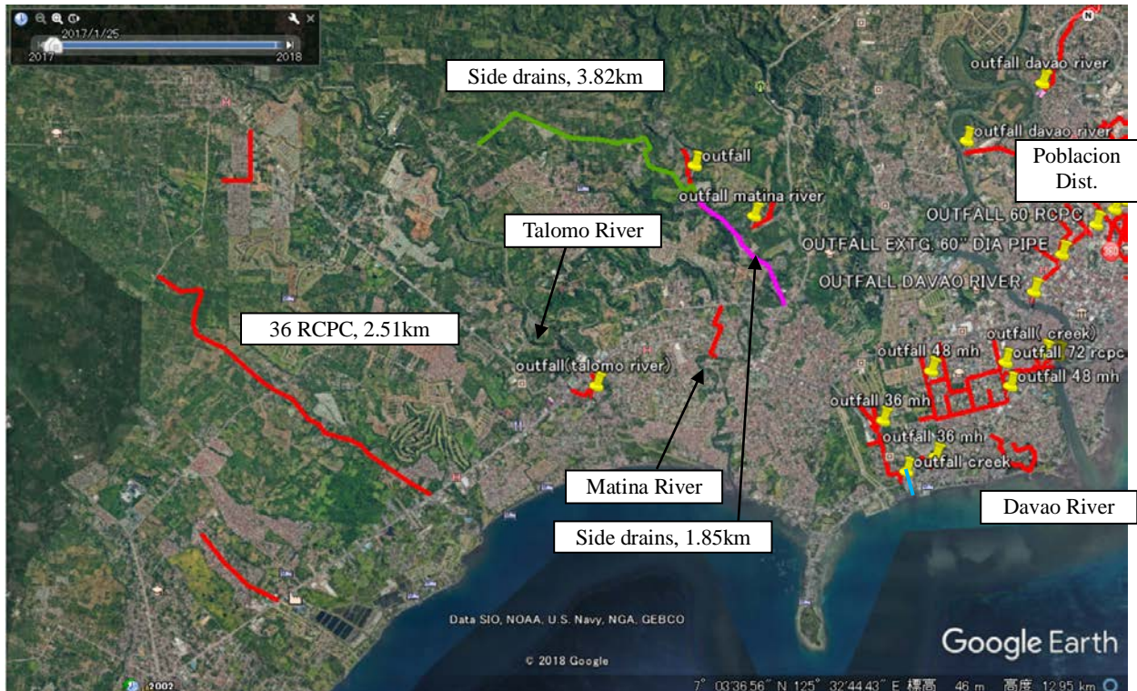
Note: Red line: drains to be developed/improved, Yellow pin: outfall to river/creeks/main drains, light blue line: creek (open channel) Source: DPWH on Google Earth image supplemented by JICA Survey Team
