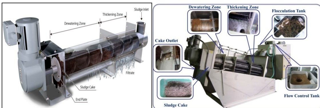
Figure 8.4.9 Energy-Saving Dehydrator (Screw Press with Multiple Layered Rings)
