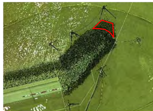
Additional breakwater in hydraulic model experiment
