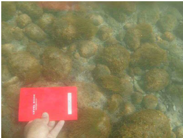
Photo 6-31 Cobble stones accumulated in the port entrance on November 29, 2017; the long side of the red Level book is 16.5 cm
