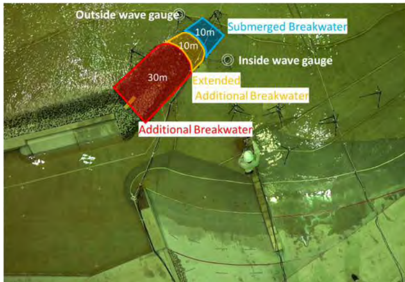
Figure 7-60 Legend of combining additional breakwater and submerged breakwater, and wave measuring points
