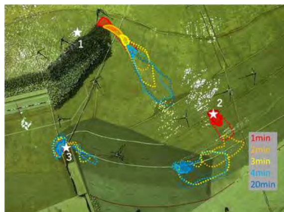
Figure 7-53 Movement of tracers after advancement of the shoreline due to the construction of additional breakwater (repost of Figure 7-52)
