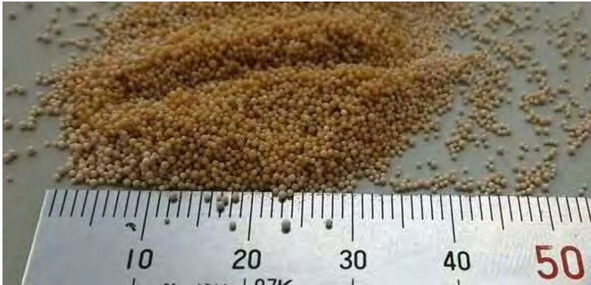
Photo 7-12 Particles of ion exchange resin utilized as tracers (Median grain size is 0.68 mm and specific gravity is 1.26)
