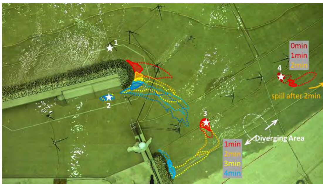
Figure 7-44 Movement situation of tracers injected at 4 points
