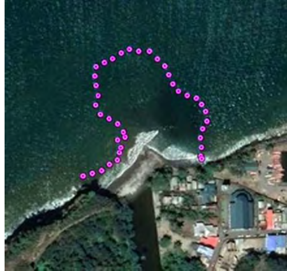
Figure 6-8 Accumulation area of cobble stones on September 3, 2018
