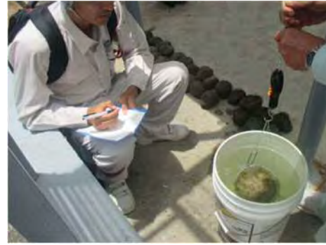
Photo 6-39 Measuring of weight in seawater
