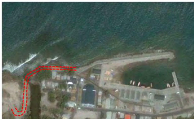
Figure 6-22 Estimated location of temporary construction road (Photo: Google Earth May 4, 2006)
