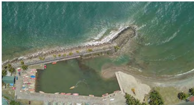
Photo 7-13 Situation that sand flows in and deposits passing through tip of groin (13 Aug., 2018)
