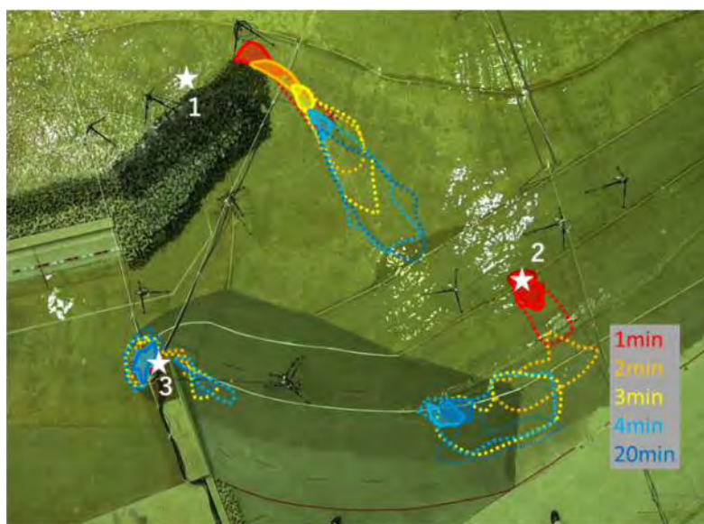
Figure 7-52 Tracer movement after advancement of shoreline due to construction of additional breakwater
