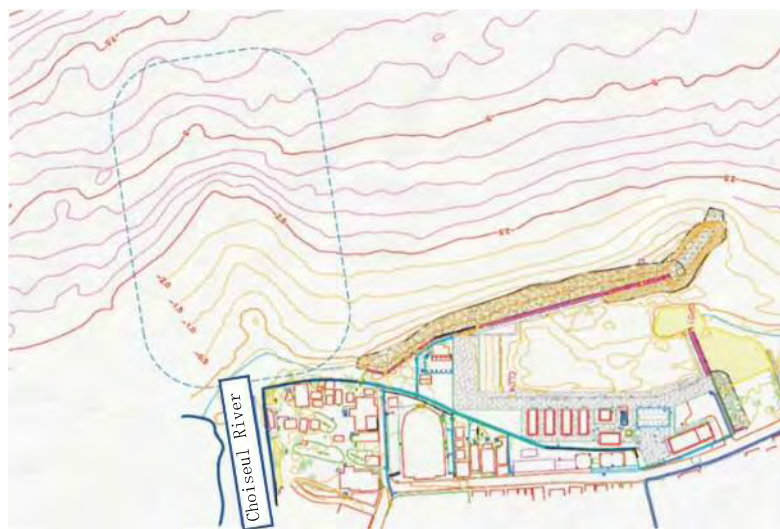
Figure 6-7 Depositional landform on the sea bottom in front of the Choiseul River mouth (Survey on November 2017)
