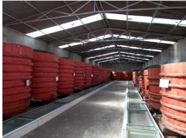
Fermenting process of fish source using wooden barrel (Van Phan Fisheries Joint Stock Company)
