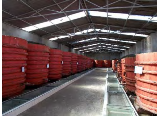
木製樽を使った魚醤発酵 / Fermenting process of fish source using wooden barrel (Van Phan Fisheries Joint Stock Company)
