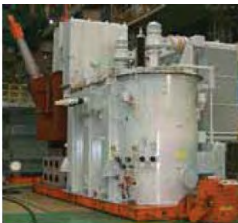
110kV-50MVA GIT (Low pressure type)
