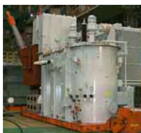
(a) 110kV-50MVA GIT (Low-pressure type)
