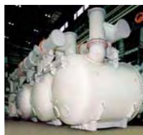
(b) 275kV-300MVA GIT (High-pressure type)
