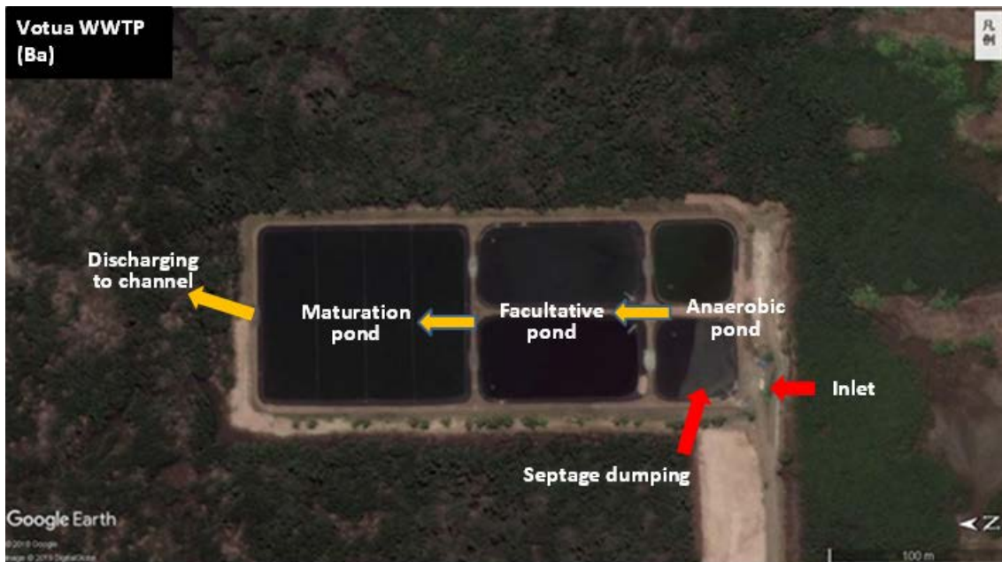
Figure 9-4.8 Layout of Facilities in Votua WWTP
