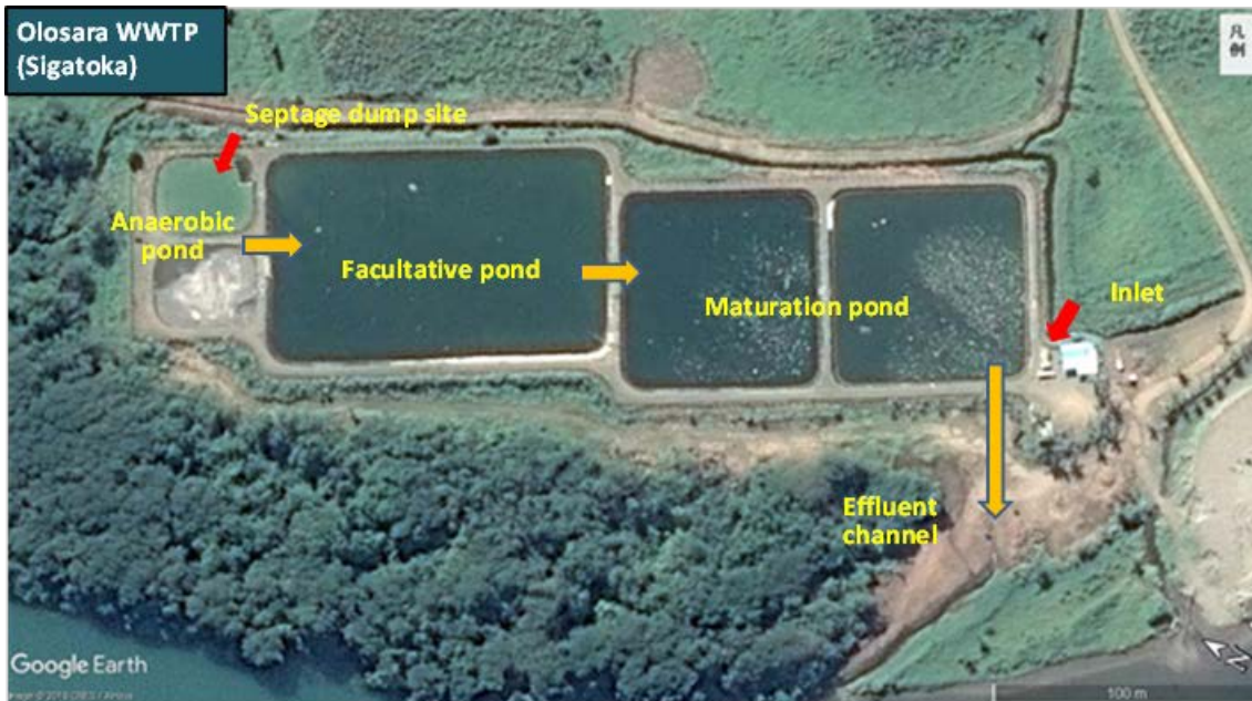
Figure 9-4.11 Layout of Facilities in Olosara WWTP
