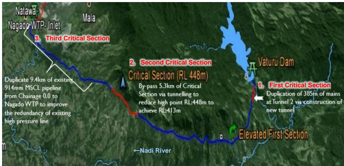
Figure 3-4.4 Measures to be taken for Enhancement of The Vaturu / Nagado Raw Water Trunk Mains
