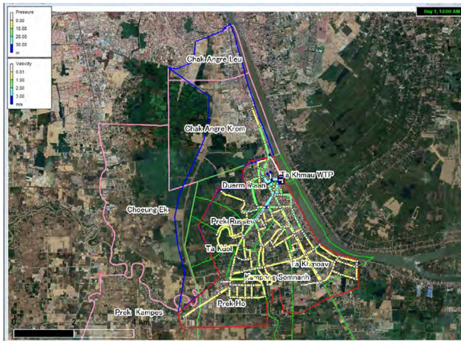
Figure A5.2 The network map and the distribution network calculation data (Pipe Network Analysis in 2024)
