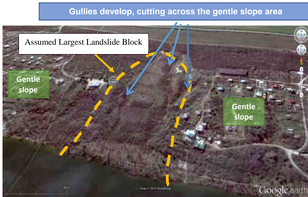
Figure 9-4-2. Landslide Block on the Right Bank on Route 2 (Google Earth Image modified by the JICA Survey Team)
