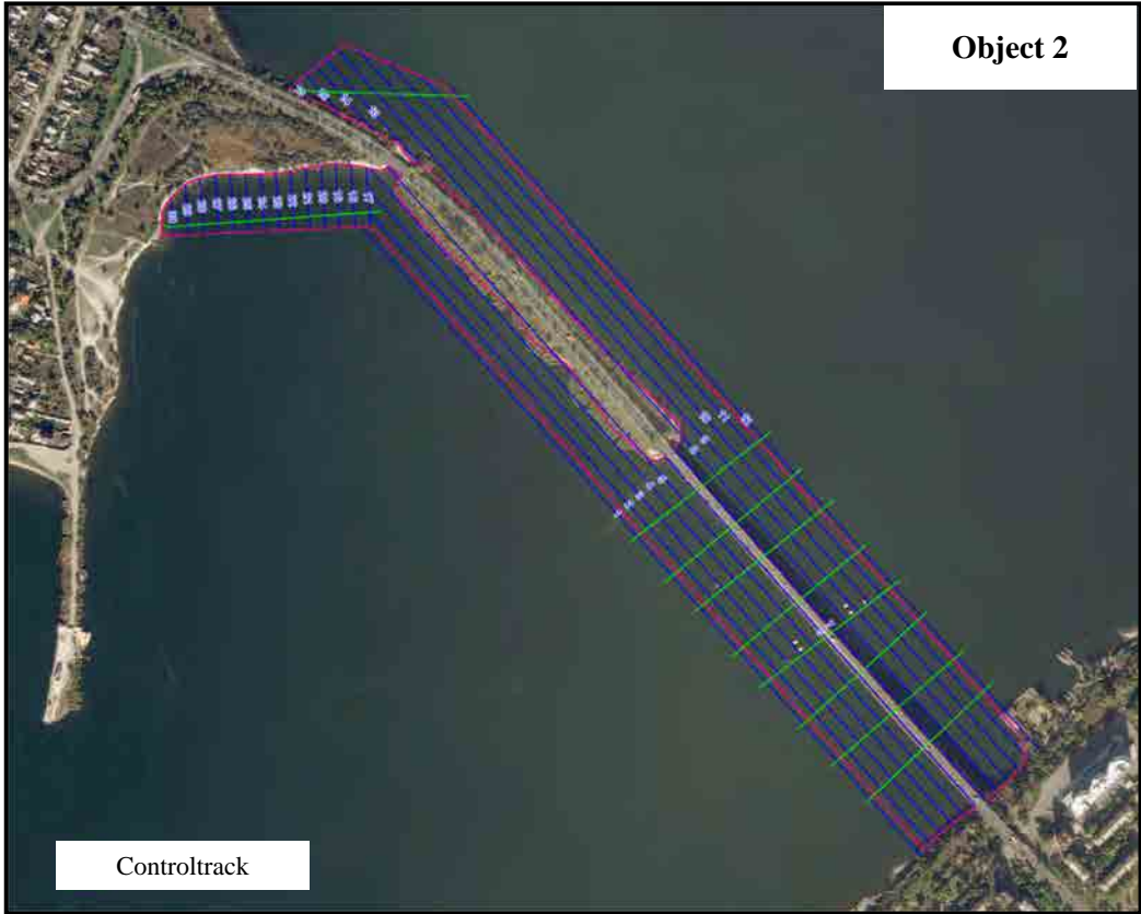
Figure 4-2-5. Layout of Survey Track Lines (Sounding Surveying)
