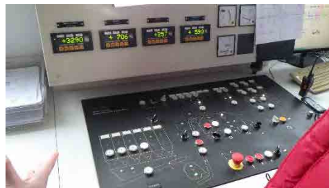
Control panel of concrete plant
