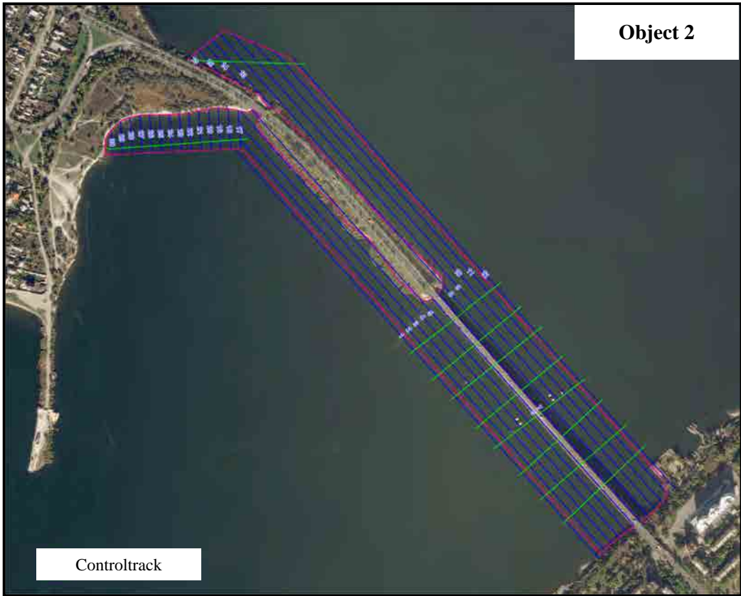
Figure 4-2-5. Layout of Survey Track Lines (Sounding Surveying)
