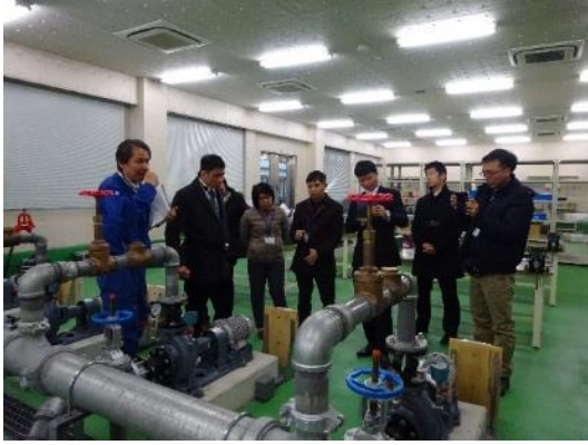
Pump repair simulation apparatus
