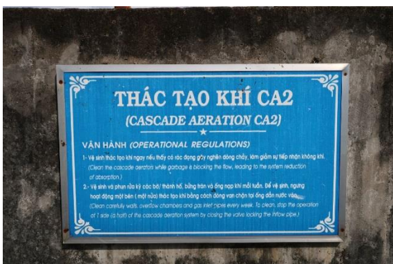
Operation regulation of cascade aeration (CA2)
