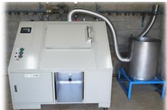
Composting plant for organic waste composting
