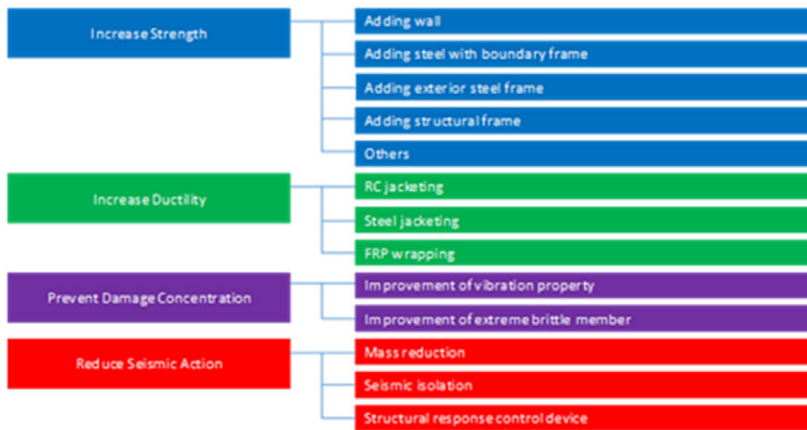
Fig. 11 Categorization of seismic retrofit methods
