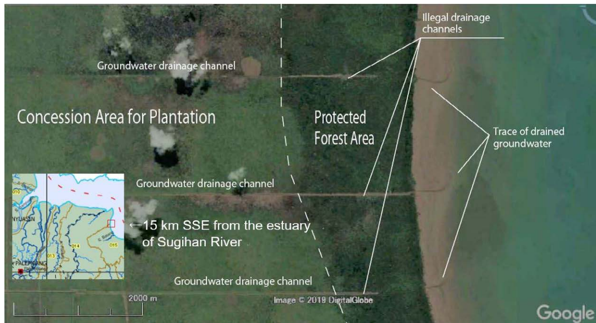
Figure 10.4.22 Illegal Groundwater Drainage from Peatland
