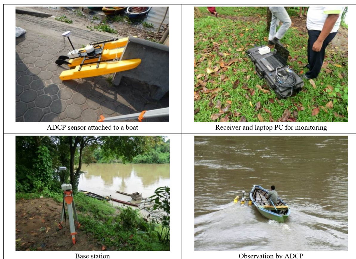
Photo 10.4.5 Discharge Measurement by ADCP
