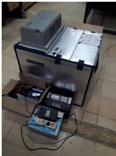
Figure 3.2. The configuration of the test (salt water, inside the building, using electric power)
