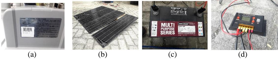
Figure 1.2. The components of the cold storage system, (a) the cooling machine, (b) the solar panels, (c) the battery and (d) the solar charge controller
