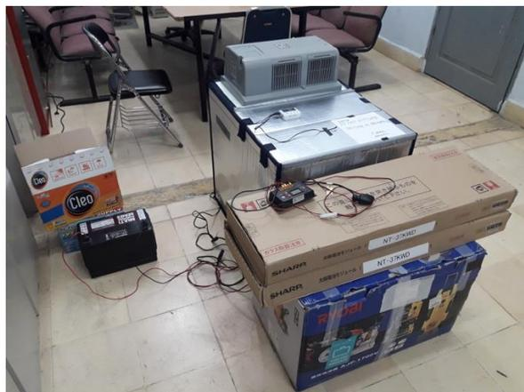
Figure 2.1. The configuration of the test (air, inside the building, using battery power)
