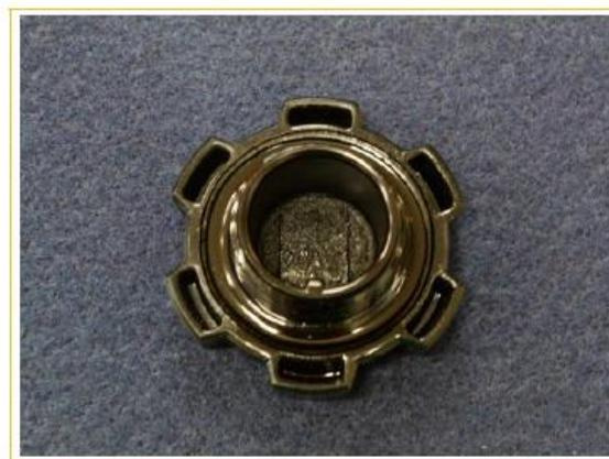
B.1.4 Some sludge present but the bottom of the cap is visible at one or more points
