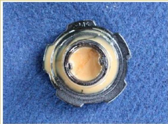
B.1.2 Thick sludge coating the inside the cap
