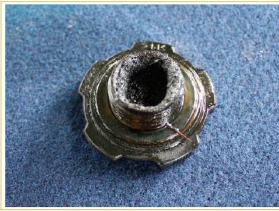
B.1.5 Small quantity of sludge visible but more than half the bottom of the cap can be seen
