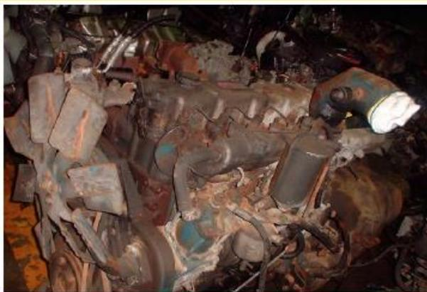
B.3.3 Examples of external corrosion at 70%
