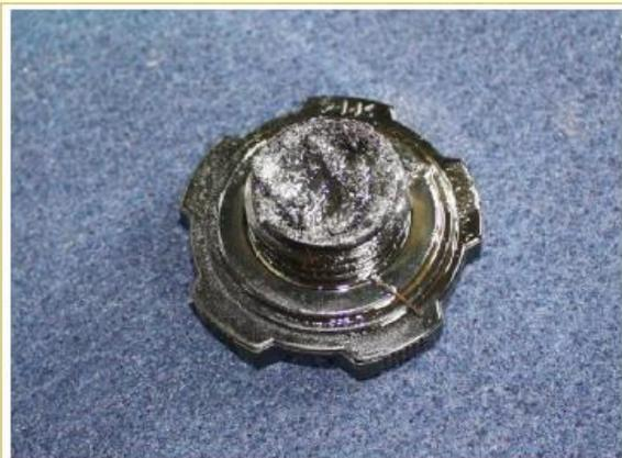
B.1.3 Quantity of sludge reduced by comparison with B.1.2 but the bottom of the cap still not visible
