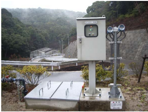
Example of measurements in the groundwater monitoring well (Automatic measurement of pH and EC)
