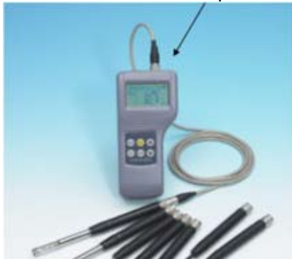
Example of equipment for measuring landfill gas generation Hot-wire current meter
