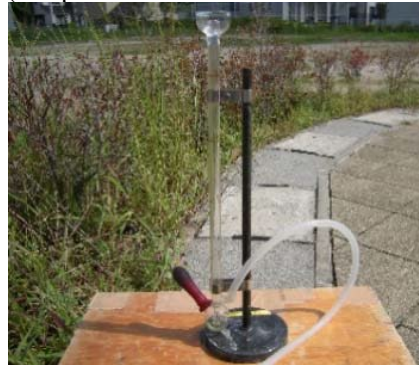
Example of equipment for measuring landfill gas generation Soap membrane flow meter
