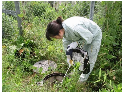
Example of measurements in the groundwater monitoring well (Simplified water level measurement)
