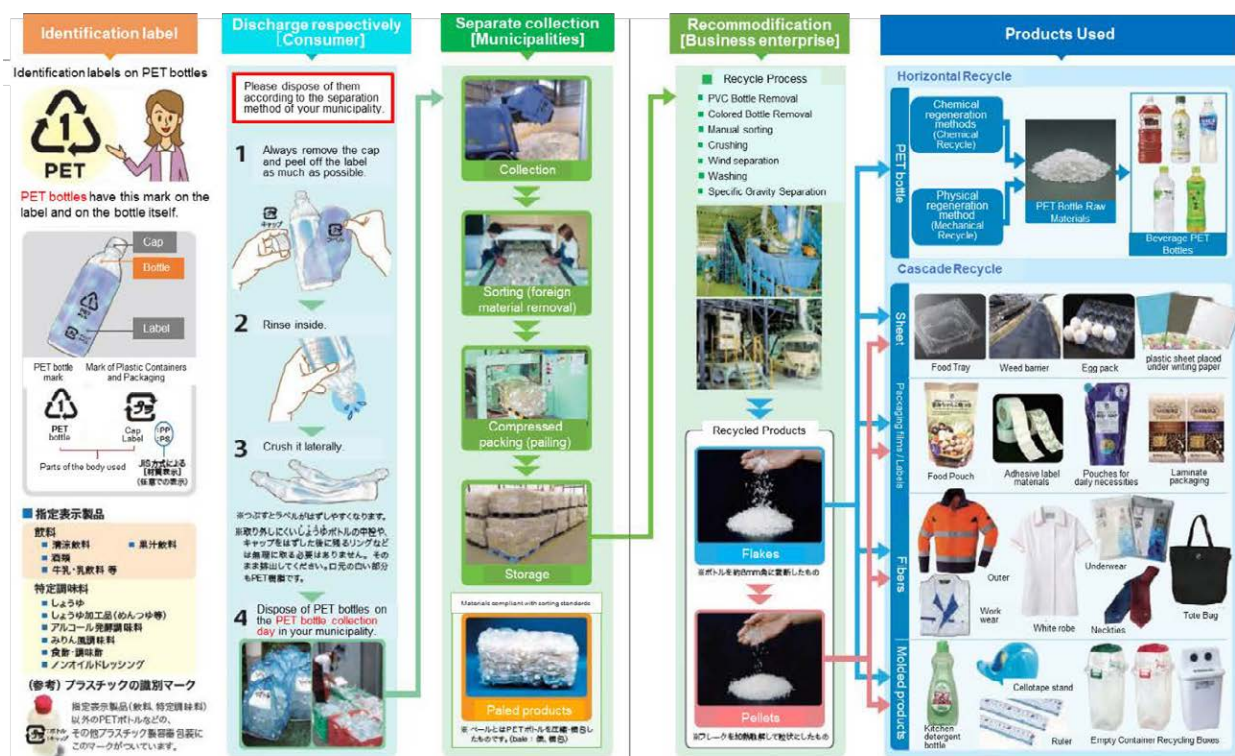
Figure 3: PET Bottle Recycling Flow
