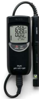
Figure 6: Portable water quality analyser
