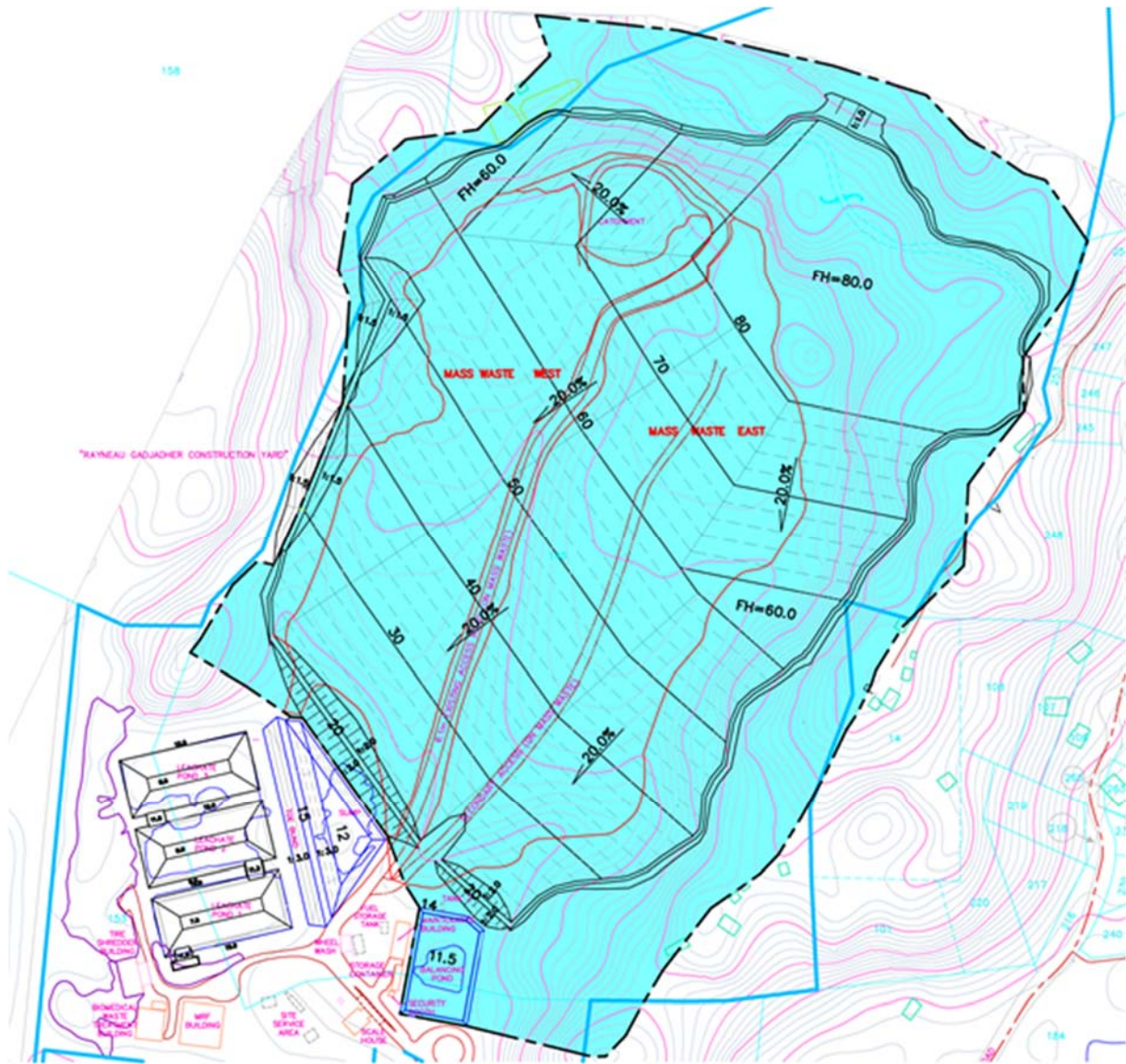
Figure 2: Catchment area for a balancing pond (16ha)
