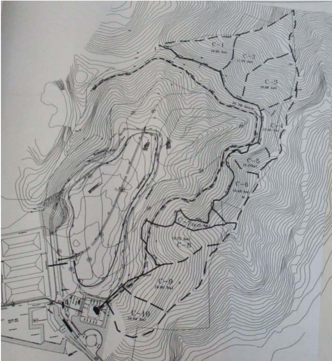
Figure 19: Stormwater catchment area (C-1 to C-10)
