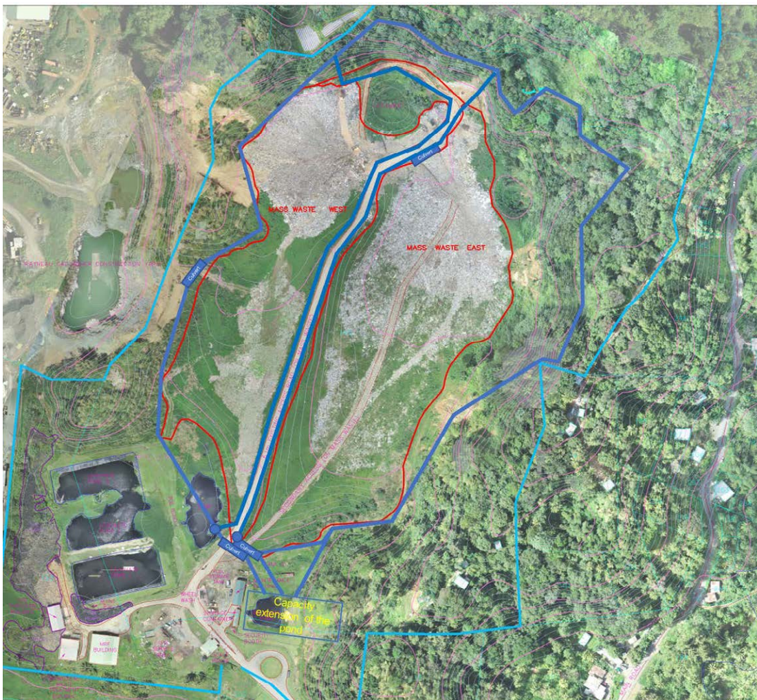
Figure 21: Storm drainage plan (dark blue line)
