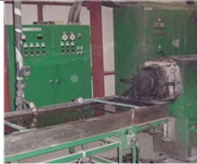
5. Granulation (1) (melting and mixing) Cold cutting
