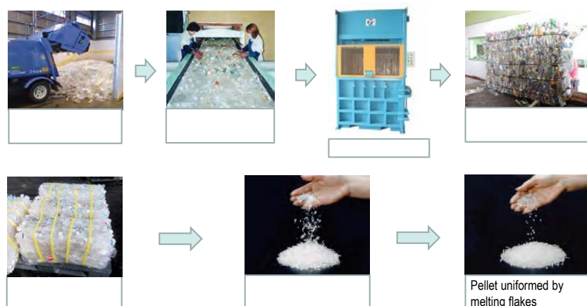
Figure 2: Flow from Collection to Flake and/or Pellet Production for Plastic Waste Recycling
