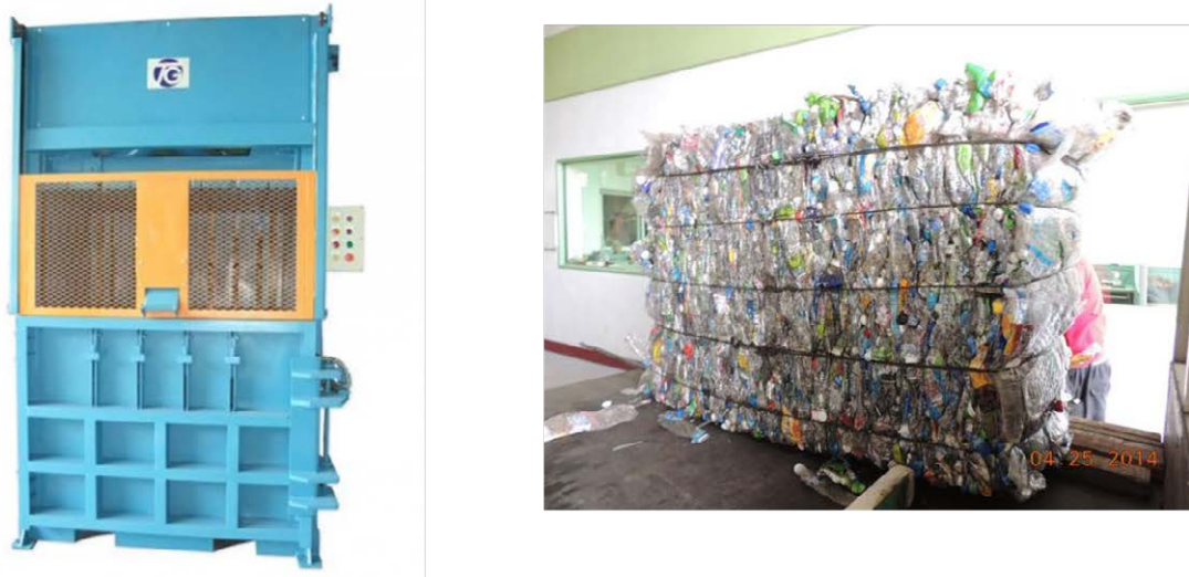
Figure 9: Vertical type baler and baled plastics
