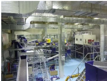
2. Pretreatment process (foreign material removal, crushing, etc.)
