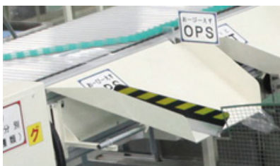
4. Material sorting Classified into OPS material, PET material, and others
