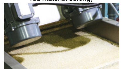
3. Material identification (near-infrared material sorting)
