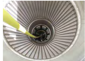
High-velocity jetting tool with centralizers hanging on high pressure hose
