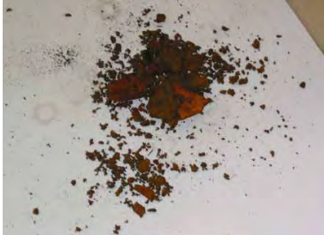
Steel pipe corrosion
