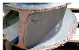
Damaged impeller from air entrainment
