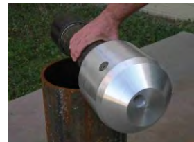
The 8-inch jetting tool (made for 10-inch wells) has four jets that are diametrically opposed and one bottom jet (Sterrett 2007).
