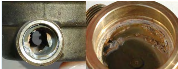
lime scale in a PD meter Limescale built-up in the inside of a single jet water meter housing
