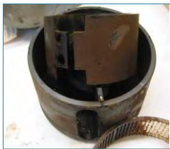
lime scale in a PD meter Limescale built-up in the inside of a single jet water meter housing
