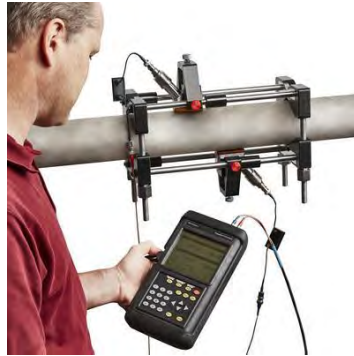
Ultrasonic Flow meter
