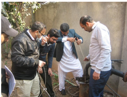
Measurement of water level at a tube well
