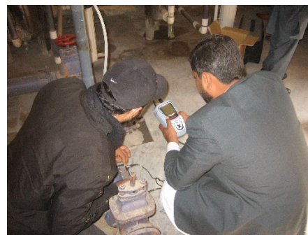
Measurement of flowrate at a tube well
