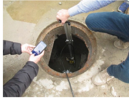
Picture 4.4.2 Demonstration of sewer camera at WASA-R
