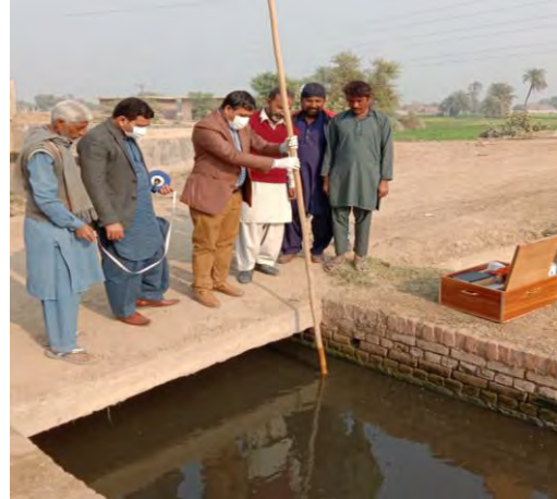
Measuring Depth of Drain
