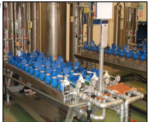
Leakage and Accuracy Test
