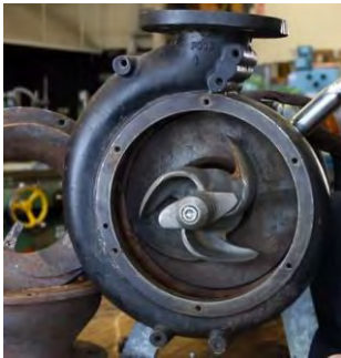
Open Impeller (Curved Blades)
