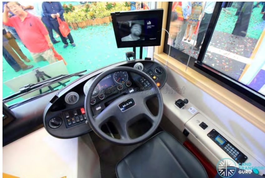
Figure A3.2.7 Fatigue Warning Systems on Singapore buses
