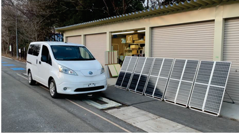
Experiment of PV and wireless charging system
