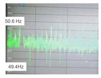
Example of frequency fluctuation with VRE
