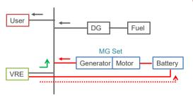
MG set is driven by battery charged from VRE and provides power with inertia → possible method to achieve 100% RE with inertia
