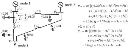
In this grid, node 1 is set as slack node, node 2 is set as P-V node, and node 3 is set as P-Q node.
