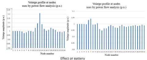
Wind turbine is located at node 13, which is north east area. Because of no measures in an estimated grid, the voltage is high. Battery is a good solution to keep grid voltages as appropriate values.
