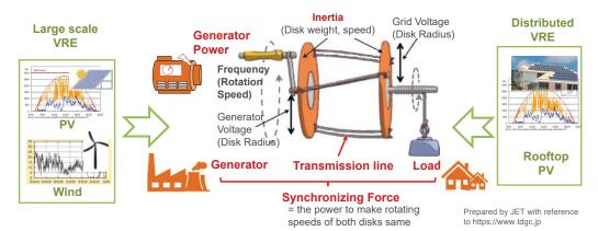
**Inertia:** The force to keep the rotation of disk when load is changed **Synchronizing Force:** The force to keep rotation speed of disks. It keeps back to the same rotation when generation power and load is varied, without entangling.
