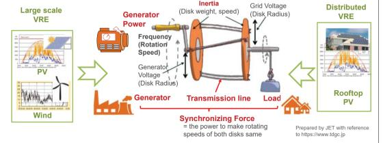
**Inertia:** The force to keep the rotation of disk when load is changed Synchronizing Force: The force to keep rotation speed of disks. It keeps back to the same rotation when generation power and load is varied, without entangling.
