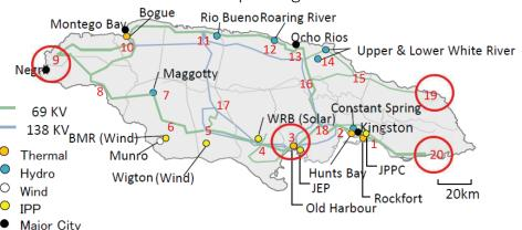
Voltages of nodes in red circle became low in the load flow analysis.
