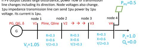
Case1 solution: PV is connected V1=1.05, V2=0.95, V3=1.08, V4=1.07 P12=1.32, P23=0.84, P34=0.57
