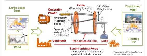
Inertia: The force to keep the rotation of disk when load is changed Synchronizing Force: The force to keep rotation speed of disks. It keeps back to the same rotation when generation power and load is varied, without entangling transmission line.
