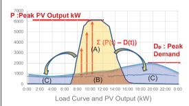
In case battery covers night load:  $P_{PV} = 6206 \text{ kW}$ PV generated E kWh = (A) + (B)Demand D kWh = (B) + (C) $\Sigma (P(t) - D(t)) = (A) > (C) / L \cdot n$  (A): Energy to be stored in Battery
