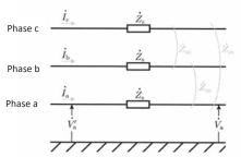
Ia, Ib, Ic: Phase Current Zs: Line Impedance Va', Va: Phase Voltage (Sending Terminal Voltage, Receiving Terminal Voltage)
