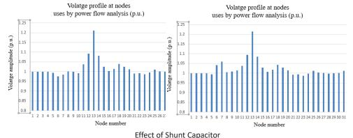
with SC in end nodes without SC in end nodes Wind turbine is located at node 13, which is north east area. Because of no measures in an estimated grid, the voltage is high.
