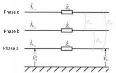
la. lb. lc: Phase Current Zs: Line Impedance Va', Va: Phase Voltage (Sending Terminal Voltage, Receiving Terminal Voltage)
