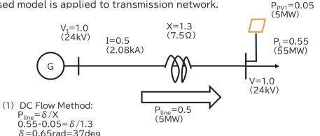
This model can be applied to extend transmission network.
