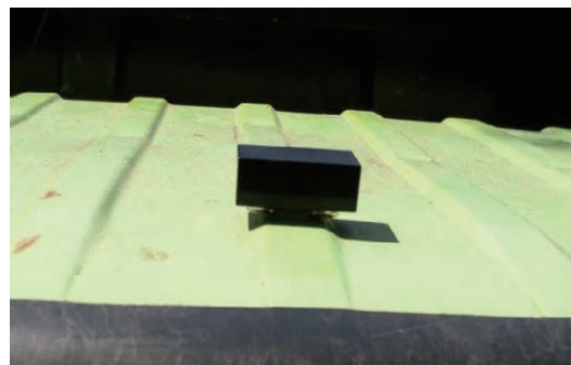
Figure 3-1 GPS Logger on the Truck
