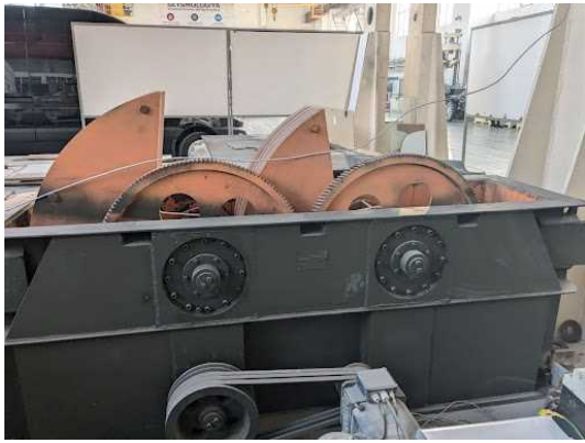
Vibration machine used on rooftops to assess the condition of buildings (Turin Polytechnic University, Tashkent Campus)
