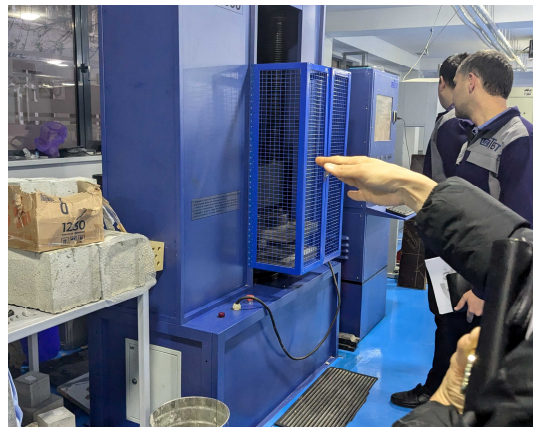
Compression strength testing machine and test piece for concrete (UzTest)
