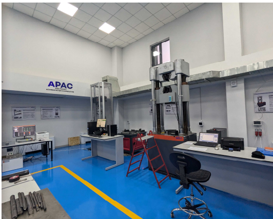
Tensile testing machine for rebar (UzTest)
