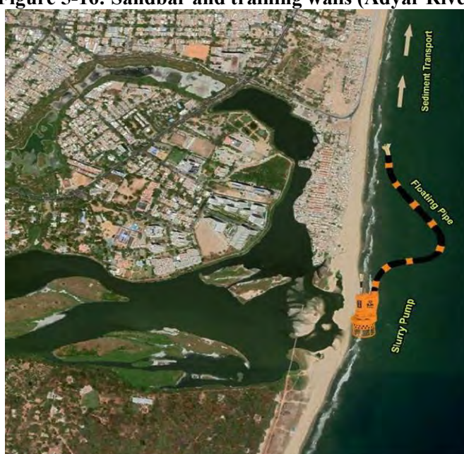
Figure 5-16: Sandbar and training walls (Adyar River)
