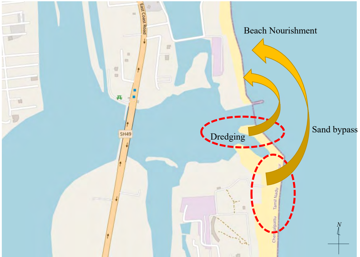
Figure 5-84: Beach Nourishment Strategy by Maintenance Dredging and Sediment Redistribution via Sand Bypassing
