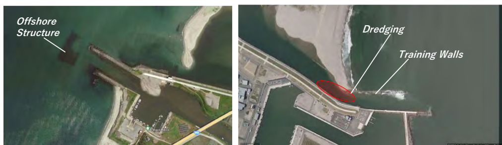
Figure 5-63: Examples of River Mouth Blockage Countermeasures in Japan (Training Walls, Dredging, and Offshore Facilities)
