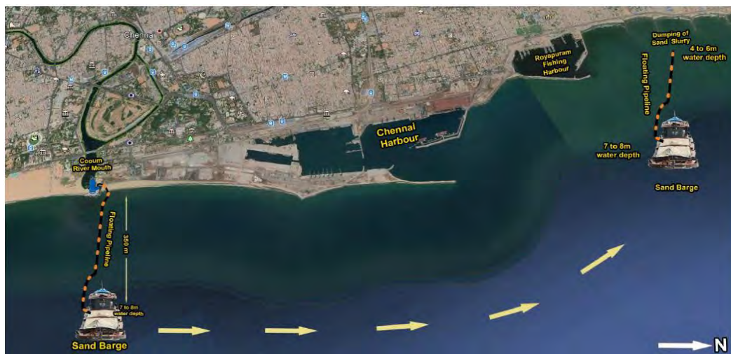
Figure 5-15: Plan for River Mouth Clogging Prevention; Dredging and Bypassing (Cooum River)
