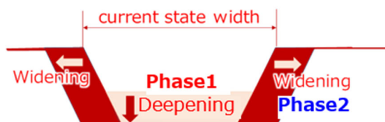
Figure 9-3: River Channelization Priority and Phases
