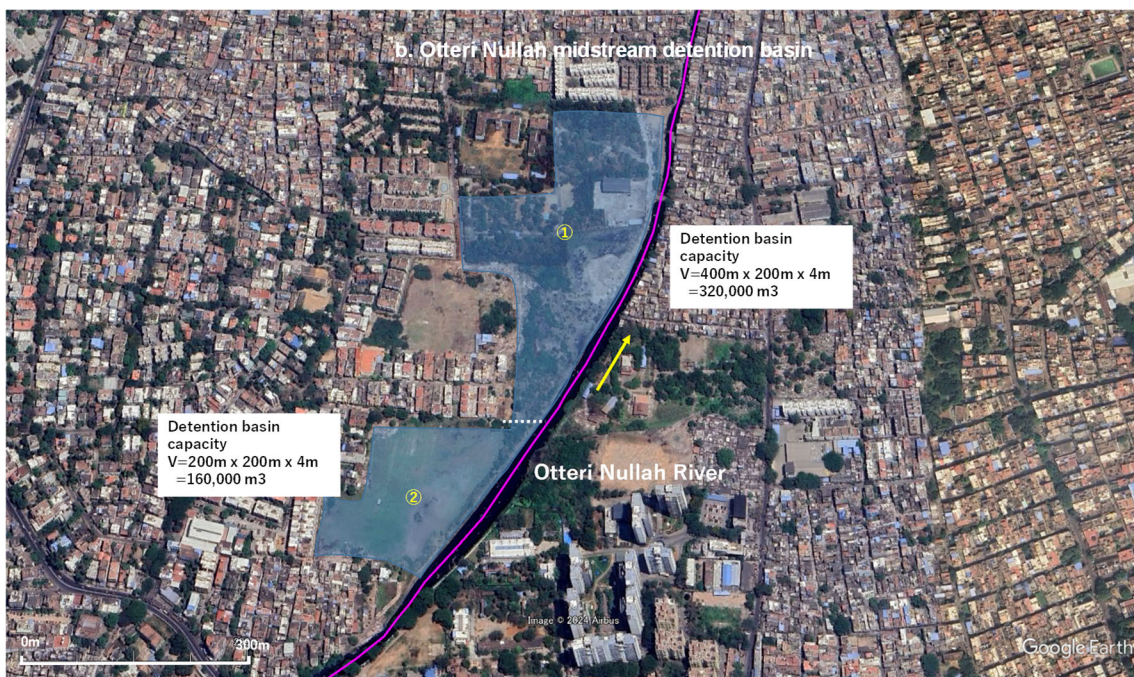
Figure 3-10: Retarding Basin Development Plan in the Midstream of Otteri Nullah The below figure shows the improvement plan for the NBC and the connected drains.
