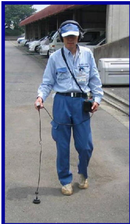
(Option) 3-Section Contact Bar with Sensor Table • Weight and Size=540g 340mm×3 Pieces (Contact Bar) φ52mm×1 Piece (Sensor Table)
