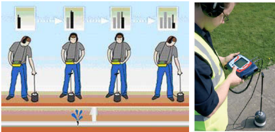
Figure 3.6.4 Survey with electronic leakage detector
