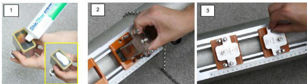
1. Add couplant onto surface of transducer as photo.
