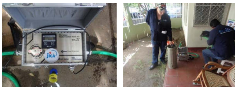
Figure 3.5.2 Example of a test meter and a standard tank
