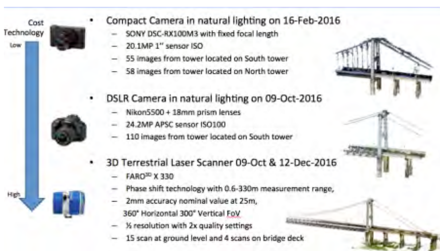
Fig.3 3D measurement of Twantay bridge using three-dimensional laser measurement and close-range photogrammetry.
