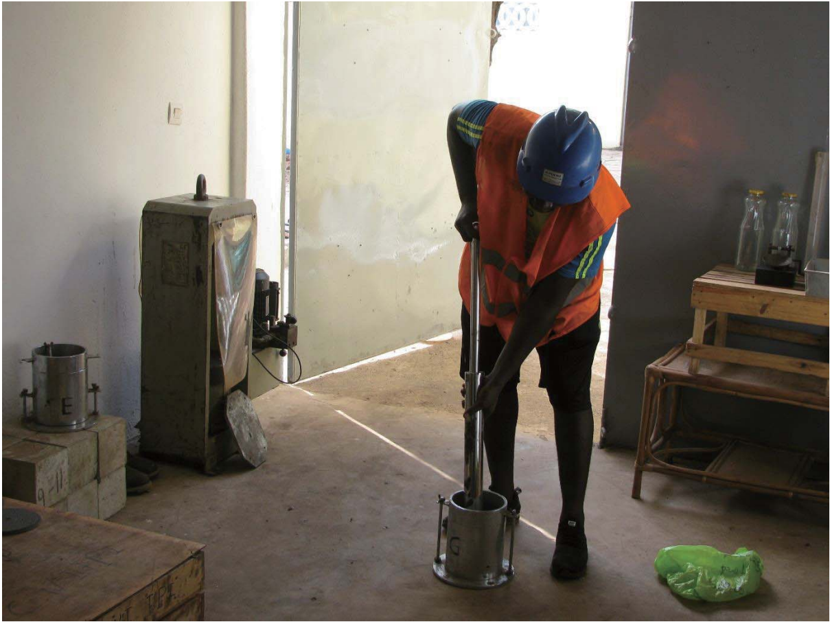
Proctor and CBR lift tests
