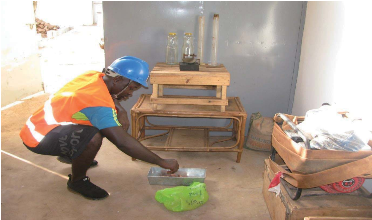
Preparation of the sample for identification tests (landfall limits, particle size analysis, water content, etc.)
