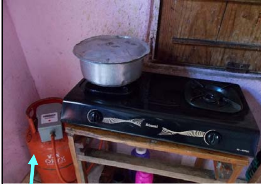
Gas Cylinder equipped with Smart Meter
