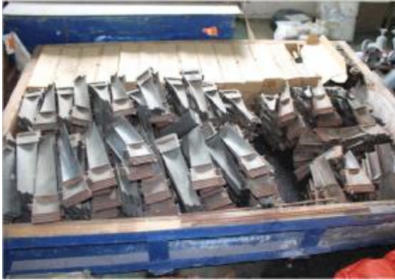
Gas Turbine Rotor Blade (Used)
