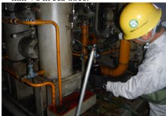
Lube Oil Sampling Sampling Point : Lube oil strainer blow line
