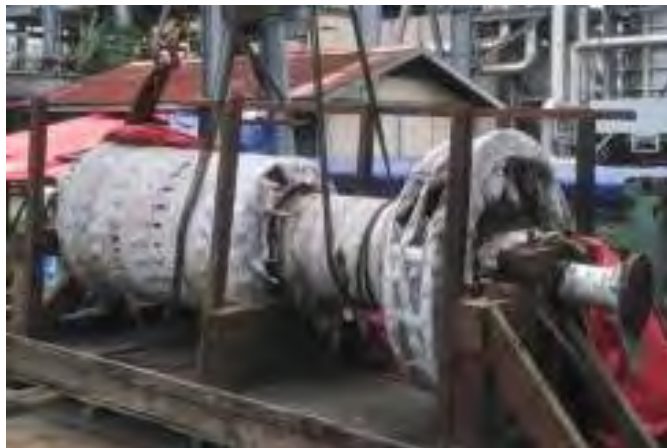
Fig. 5-16 Spare Rotor That Was Installed After Compressor Damage
