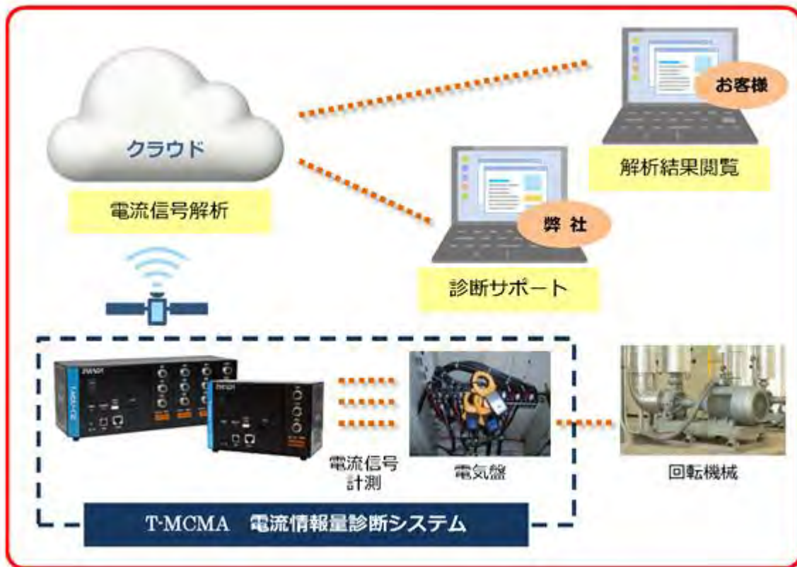
Fig. 6-6 Configuration Example of a Rotary Equipment Diagnostic System
