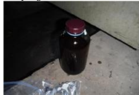
Lube Oil Sampling Sampling Point : Lube oil strainer blow line
