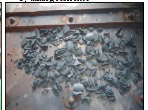
Damaged parts found in gas turbine
