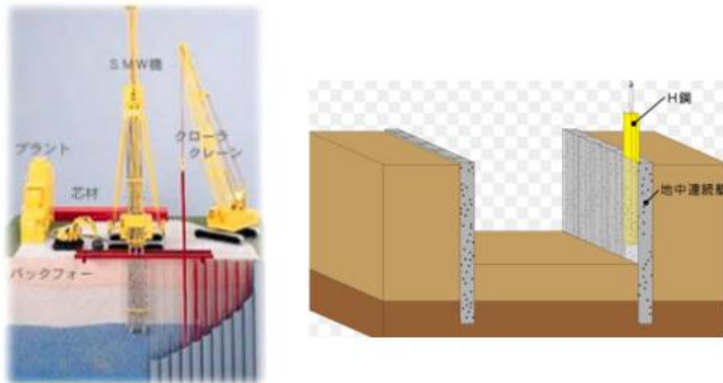
Figure 14-22 Explanation of SMW (Soil Mixing Wall)
