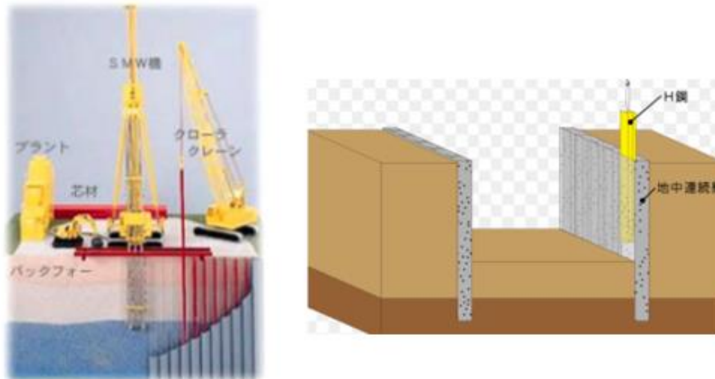
Figure 6-23 Explanation of SMW (Soil Mixing Wall)
