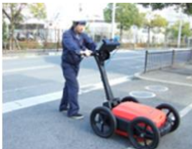
Figure 14-26 Picture of GPR survey
